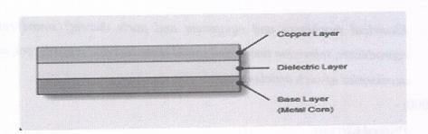
Here, MCPCB consist of 3 layers i.e. a metal base on which circuit needs to be formed but to make the circuit electrically non-conducting in respect of metal base, a very thin di-electric material is used to separate two metallic layers to avoid electric failure of circuit. Further, the thickness of above mentioned 3 layers, as mentioned in the submission by Dr. Kishore Chatterjee. Professor, IIT Powai, are as follows:
